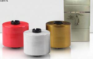
**EkoTear** is made up of a **23micron**, single ply, **PET film containing 90% post-consumer recycled (PCR) content.** coated with an **acrylic adhesive system** and a **silicon release coating**. This high tensile tear tape offers **good initial tack**, **excellent shear resistance**, **and strong ultimate adhesion**.
