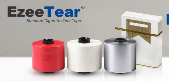
**EzeeTear** is manufactured from a specialized grade of **23-micron monoaxially orientated polypropylene (MOPP) film** coated with an acrylic adhesive system and a silicon release coating. This high tensile tear tape offers good initial tack, excellent shear resistance, and strong adhesion.
